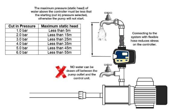
Note: The controller provides dry-run protection in both modes.
